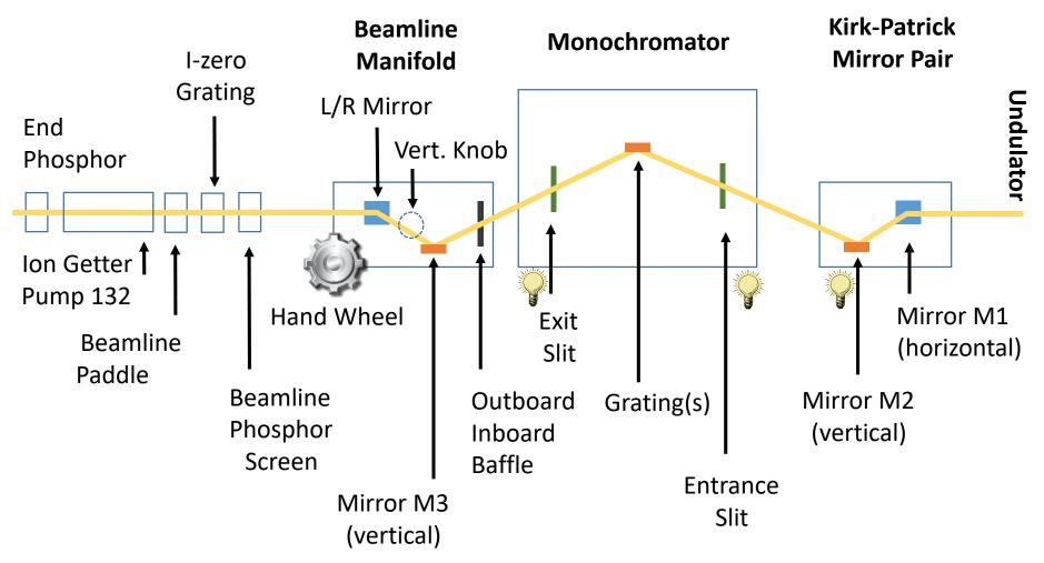
Beamline range: Low Energy Grating goes from 18 to 75eV (can technically go up to 92eV but is not reliable in this range)
