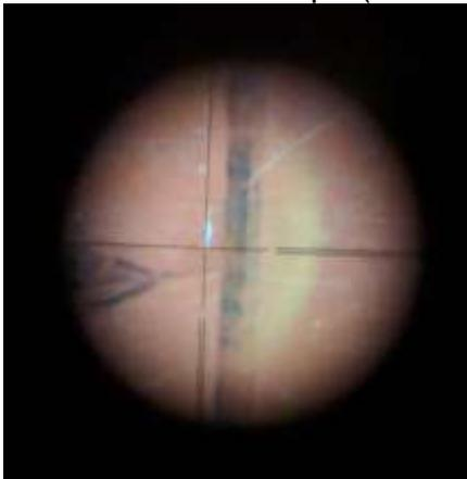
**Image 4:** Sharpy marks for beam on floor at beamline 10.0.1.3. Near target = 2<sup>nd</sup> closest to the telescope (~ 1.5m) used as the near target in Step 4): see image 6.
