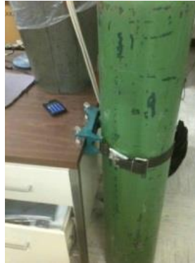
Combustible strap only and questionable "clamp"
