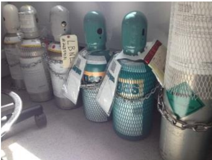
One chain for small cylinders
