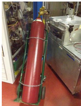
Unsecured (cart not secured)
