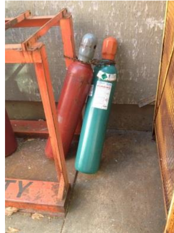
Not upright or properly secured
