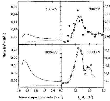
Figure 5. Ratios of transfer ionization to capture probabilities as function of the H transverse momentum. (10)
