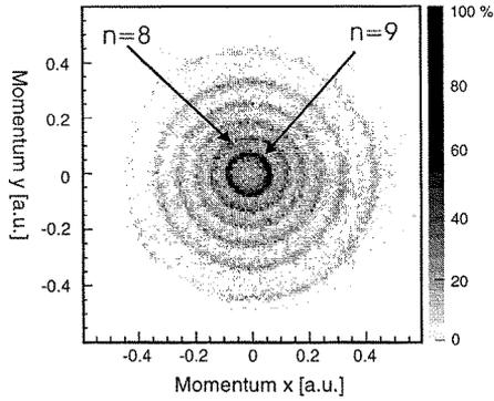
Figure 3. electron momentum distributions for autoionization processes close to the double-ionization-threshold for the reaction  $\text{He} + \gamma \rightarrow \text{He}^{**}(m, m') \rightarrow \text{He}^{1+}(n) + e_{Aug}$  (9). x and y are oriented perpendicular to the polarization vector. In order to reveal the rings that are visible in the plot a narrow cut in z-direction at  $z=0$  was applied.
