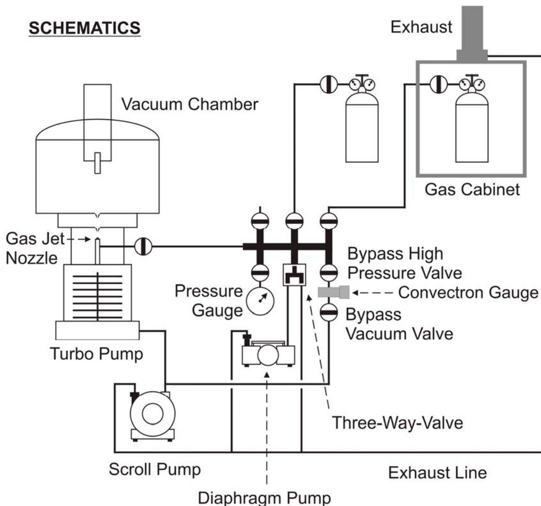
**Picture of the Gas Manifold:**
